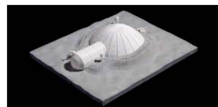
The overall sectional dimension could be in the region of 10m by 5m. The overall shape of the inflatable has continuous curvature so that it can withstand the internal pressures. This inflatable does not give any protection, besides providing an atmospheric pressure and conditioned space. It is quite obvious that such a fragile structure would have very limited rigidity and will need to be protected.
