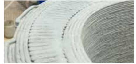
Fig. 5: Design explorations of different tool path options.
