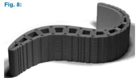
Creating the tool paths in a parametric model was not sufficient as it did not visually represent the design. Therefore each of the tool paths had to be converted into extrusions. This model was then also 3D printed through with a Z Corp. printer.
