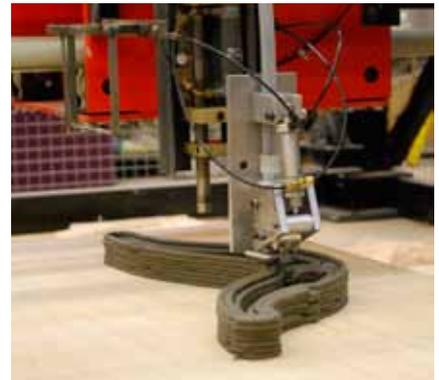
**Fig. 3:** Wall section with cavities that can incorporate services and locally optimised insulation and reinforcement.
