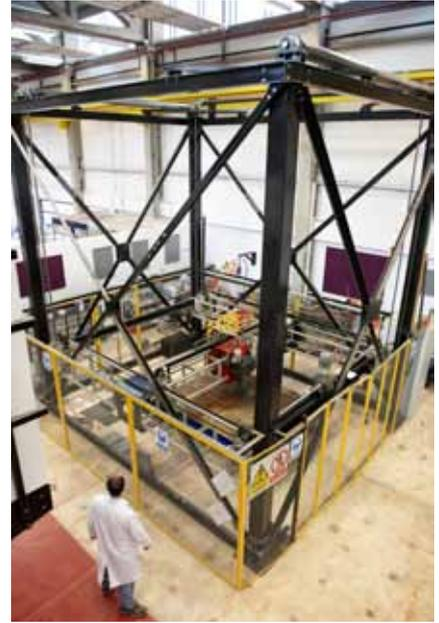
**Fig. 2:** The large computer controlled 3 axis steel gantry system deposits concrete with high precision.
